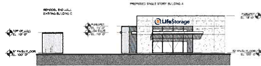
A1 WEST FRONTAGE ELEVATION BUILDING A SCALE 3/32" = 1'-0"
