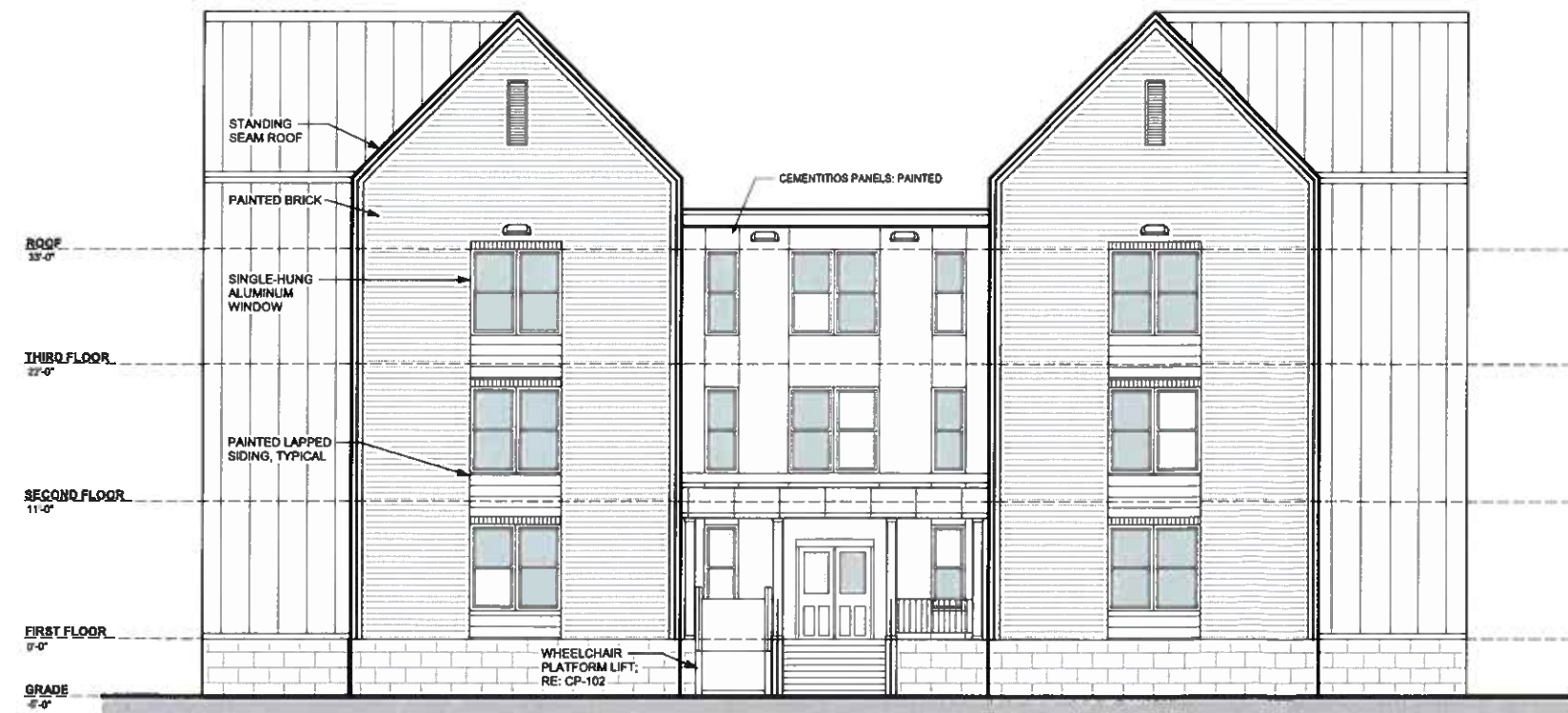
3 ENLARGED EXTERIOR ELEVATION - PARKING LOT 1/8" = 1'-0"
